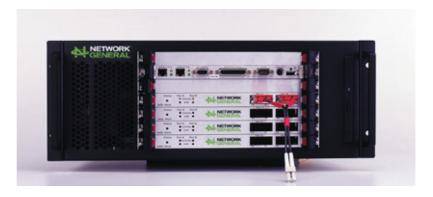
The Network General s6040 provides Sniffer Distributed functionality for the network core.
