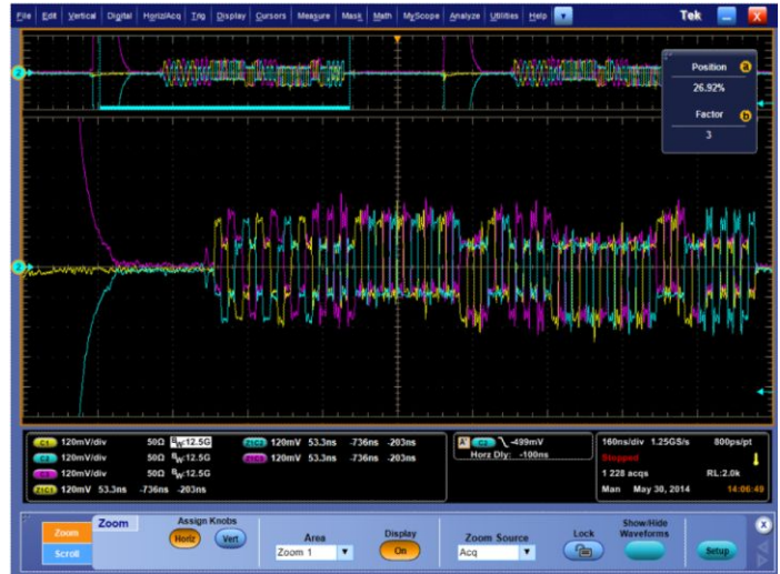
C-PHY Signal Capture on an oscilloscope
