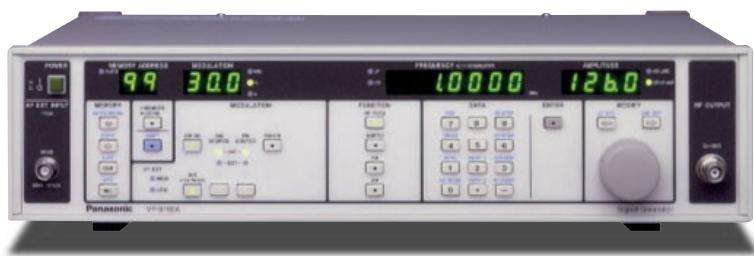
A high purity signal source with output level of 126 dBμV [emf], it's coverses the broadcast bands with its wide 100 kHz to 140 MHz range.
