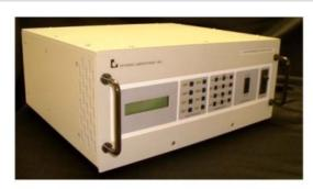
The OL 16A, 65A and 83A are microprocessor controlled, precision DC current sources specifically designed to accurately operate tungsten filament lamp standards and calibration sources. The power output range is 10 to 100 watts for the OL 16A, 10 to 200 watts for the OL 65A and 10 to 1000 watts for the OL 83A. All three units feature:
