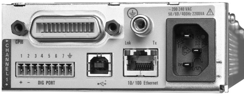
Figure 1. Connectivity: GPIB, 10/100 Base-T ethernet, and USB 2.0 all standard
