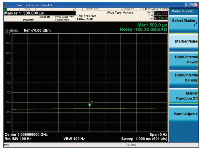
Figure 5b. At 1 GHz center frequency, an MXA shows -165.38 dBm DANL normalized to RBW of 1 Hz, with the preamplifier on.
