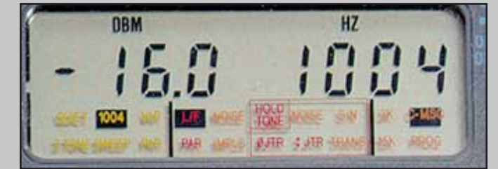
Large easily-read LCD with simultaneous display of test set-up menu and measurement.
