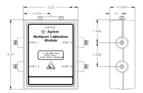
The N4430A 4-port ECal module is the perfect companion for Agilent's balanced measurement solutions. Fast, and easy-to-use, this ECal module replaces the standard SOLT-based mechanical calibration kit with a solid-state transfer standard.
