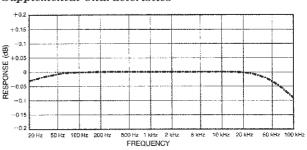
Typical flatness of source and analyzer combined (source voltage set to 1 V, 1 kHz reference).
