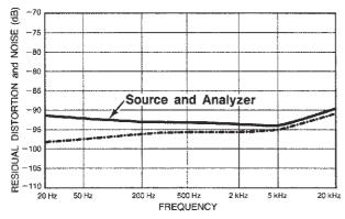
Typical residual distortion and noise of the source and analyzer combined (source voltage set to 1.5 V, 80 kHz BW). Dashed line represents typical residual distortion and noise for the analyzer only.
