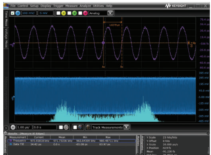
Use Infiniium Offline to find signal anomalies, such as power supply coupling.
